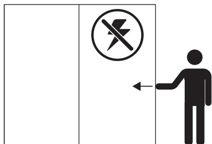
In the event of a power failure, the doors may also be moved manually, though more force will be required due to the friction and resistance of the electromechanical system.
