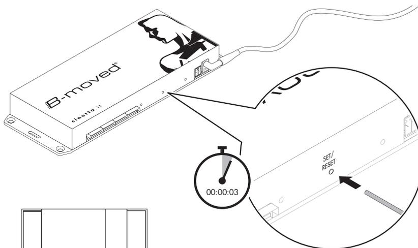
Activate the function for automatic detection of door track limits, as described in Section 2.3, by long pressing (3 seconds) the 'SET/RESET' button on the control unit. One door at a time, starting from the first door to the left of the cabinet, the doors will move slowly towards their respective track limit stops.
