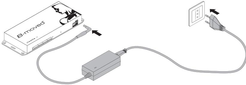
After checking the correct connection of the motors to the control unit and bringing the doors to their closed positions, the control unit can finally be powered via the power supply unit.
